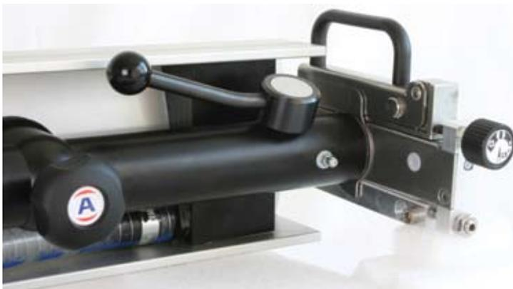
*Image left: The optional NOVA Compact suspension system offers possibility of on press service and maintenance. The chamber is simply pulled back to service position, the rotation brake is released and the chamber is rotated to an upward facing position. End-seals and doctor blades can then be easily changed.*
