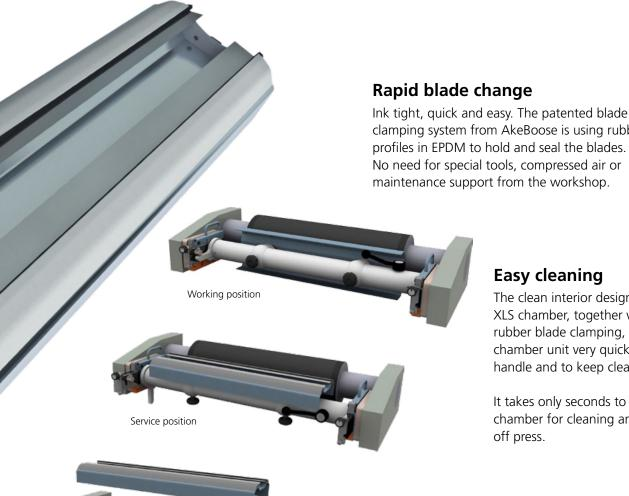
clamping system from AkeBoose is using rubber profiles in EPDM to hold and seal the blades. No need for special tools, compressed air or maintenance support from the workshop.
